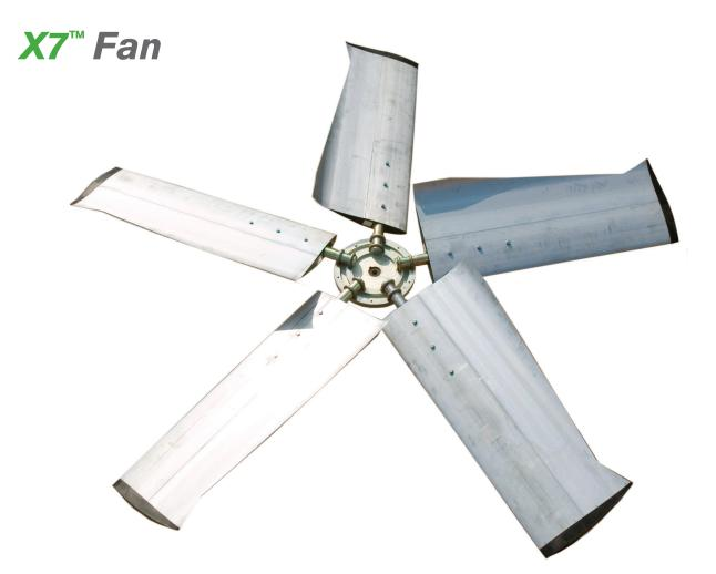
The Marley<sup>®</sup> X7 fan is designed for induced-draft cooling tower applications, offering distinct advantages over other fan designs. The Marley FlareTip<sup>™</sup> blade enhancement provides increased performance overcoming tip clearance losses—aiding the movement of air next to the fan cylinder.
